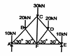
(d) Determine the magnitude and nature of forces in the members of truss shown in figure by method of joints.
