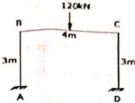
(b) Analyze the portal frame loaded as shown in figure by Moment distribution method. Draw BMD.
