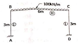
(c) Analyze the portal frame loaded as shown in figure by Moment distribution method. Draw BMD. Take EI as constant.
